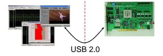
Any block, designed with C/C++/System C, MATLAB Simulink, or RealView Soc Designer, can be replaced with HDL-based circuit on SIMIMS FPGA solutions.
