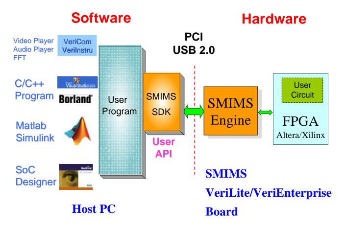
All PC peripheral devices become I/Os of your circuit. All PC software blocks can co-work with your circuit.
